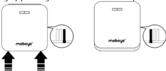
Insert the SIM card into the module.
