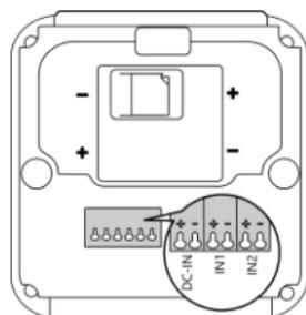
As default the input is programmed as Normally Open (NO) contact. This means the input is triggered if the input is closed for at least 1 second. In case the contact is Normally Closed (NC), see paragraph 5.8. If the sensor needs to be activated for a longer period before triggering an alarm, see 5.8.
