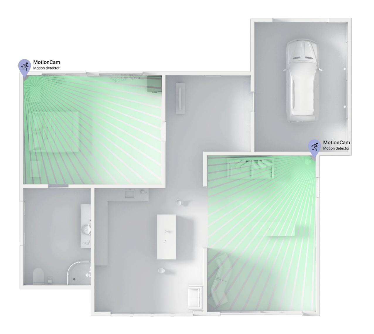
MotionCam should be installed in locations where one needs to see what has triggered the alarm.
