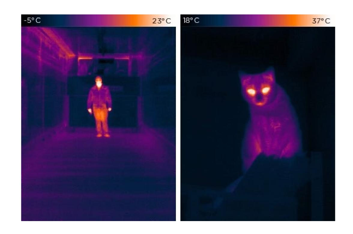
The closer to white, the stronger the radiation (the warmer the object). The closer the object is to the detector, the larger the heat spot is.
